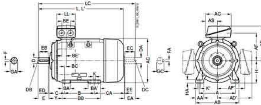
Types of construction **IM B5 and IM V1**
