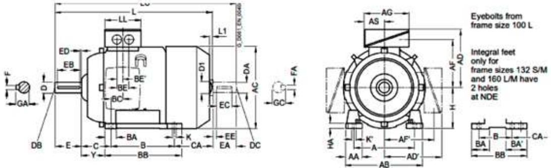
*Types of construction IM B5 and IM V1*
