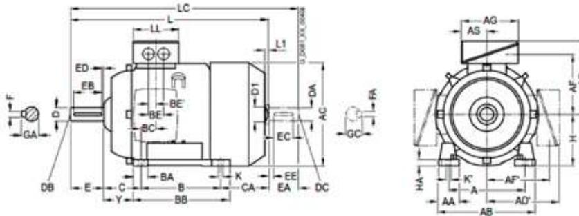
*Types of construction IM B5 and IM V1*
