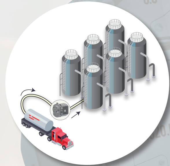
Unloading from truck to storage silos for various product range
