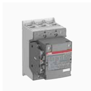
07 Line contactor AF - Isolation at stop - Isolation at faults - Emergency stop - Back-up DOL starter
