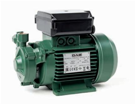
Pump body, motor support and impeller in brass. Carbon/ceramic mechanical seal. Stainless steel motor shaft. Asynchronous, closed motor cooled by external ventilation.
