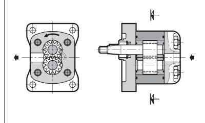
The 1P pumps are fixed displacement external gear pumps with axial clearance compensation.
