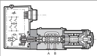
The DXJ3 valve is a four-way servo-proportional valve where the spool moves inside a sleeve. This valve has a direct drive with a linear force motor resulting in high dynamic performances which are independent of system pressure. The spool position is controlled by a linear transducer (LVDT) with closed loop which ensures high
