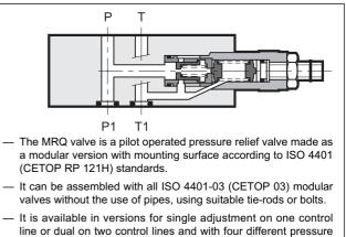
adjustment ranges. — This valve is normally used as a hydraulic circuit pressure
