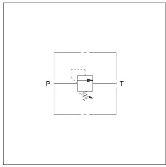
CD1-W DIRECT OPERATED PRESSURE CONTROL VALVE SERIES 10
