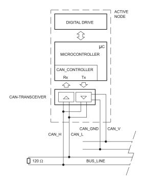
N.B. : insert a 120 Ω resistance on pin 4 and pin 5 of the CAN connector when the valve is the closure knot of the CAN network.
