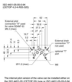
(R05) type of mounting interface (ports X and Y of the latter version are not to be used).
