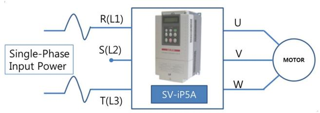
Figure-3 Terminal Wiring Diagram
