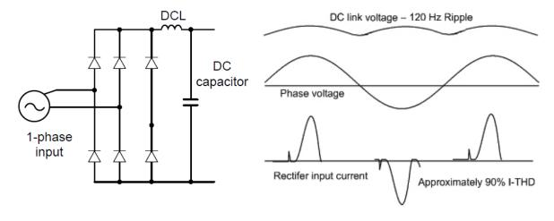
Figure-2 Typical Single-Phase Configuration
