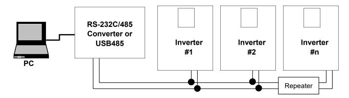
\* REPEATER is not a required item but helps communication in long-distance communication or high noise environment.
