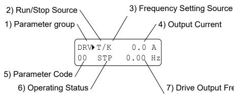
6) Operating Status / 7) Drive Output Frequency During Run, Command Frequency During Stop
