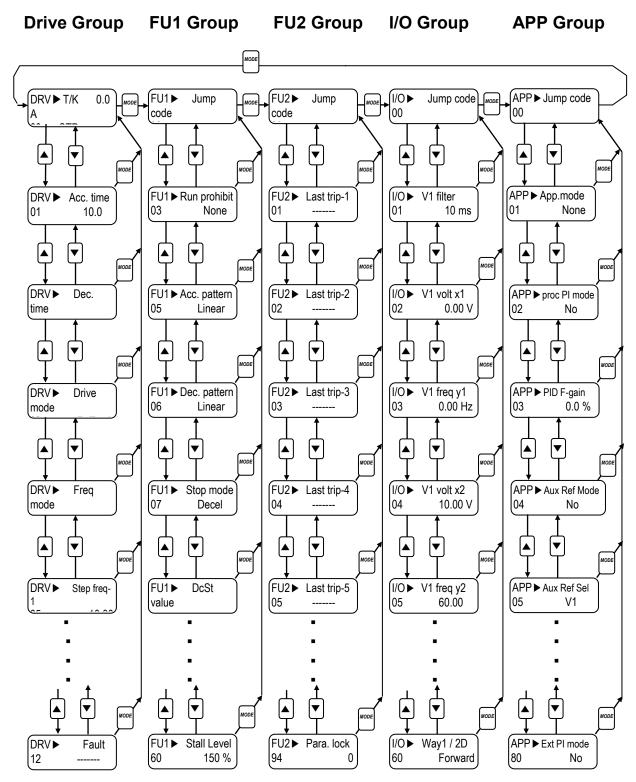
**► Note:** This figure shows the group and code navigation through LCD display keypad. It can be different from the actual display due to the group addition or code change.
