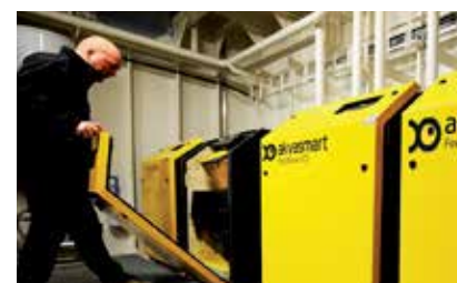
Inspection of a Feed Blower installation, noise cabinets with easy access.
