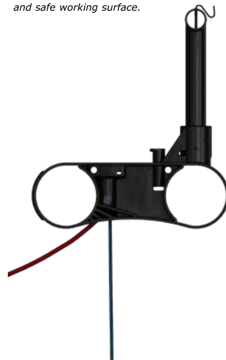
All the weight of the net and sinker tube system is supported by the floating pipe - NOT by the handrail.
