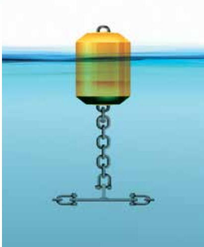
All ropes are connected to the mooring plate well below propeller depth, ensure easy boat access around the cages.
