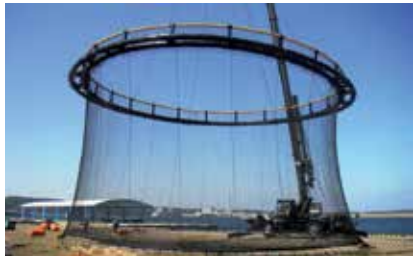
The upper section of the EcoNets have slightly tapered vertical walls with a 1m jump-net up top and the bottom is normally cone shaped.
