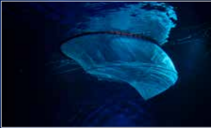
Net in 1.5 knot current
