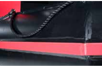
Polarcircel RBB hulls are self-bailing and have rigid pontoons filled with polystyrene that makes them virtually unsinkable.
