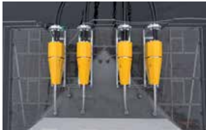
Feed Selectors can easily be installed at the front or the side of the barge.
