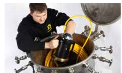
Cameras, cables and connection plugs are pressure tested to ensure that the equipment is 100% water proof.
