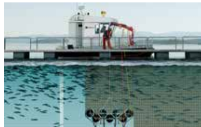
The hard non-fibre wire reduce settling of marine fouling and makes the net easy to clean with a net cleaner from AKVA group.
