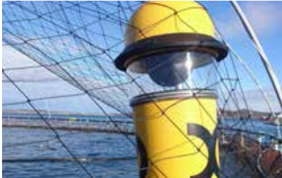
The CAP has a built-in surface camera for monitoring fish surface activity and feed spread even in difficult light conditions.
