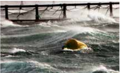
The bouys are made of rotation moulded polyethylen filled with polystyrene foam. This retain full floating capasity even if the shell has been damaged.
