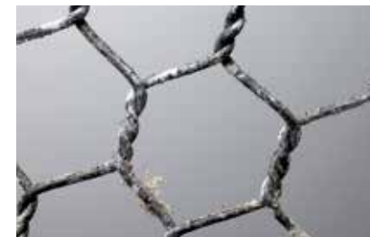
Net sample after 20 years use in seawater in Japan. High tensile strength is retained.
