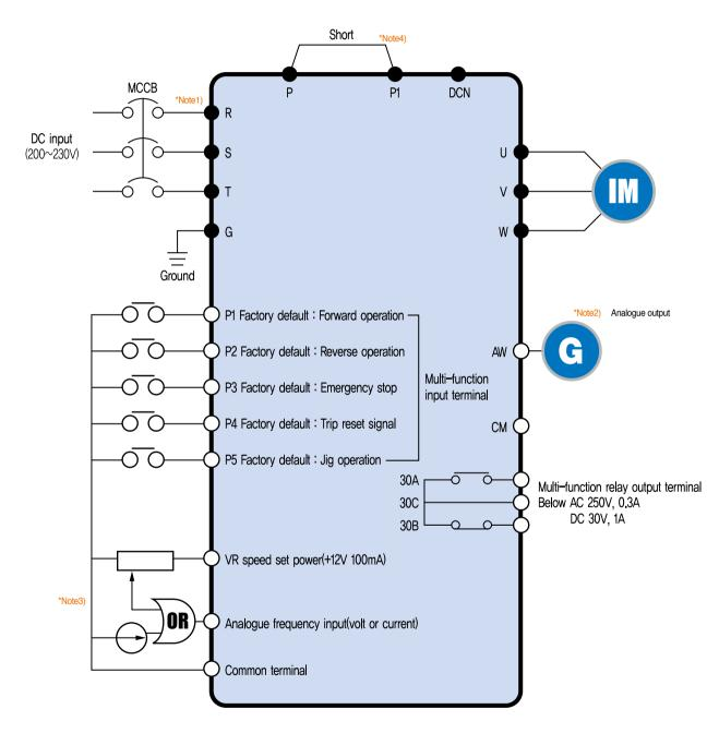
"Note1) " • "and " o "means the main circuit and the control circuit respectably.
