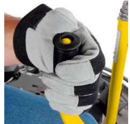
A thumb button on the steering lever controls the water spray system on BG740 and BG910.
