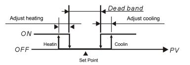
Output of defined when in PID control mode (Ctrl = PID):
