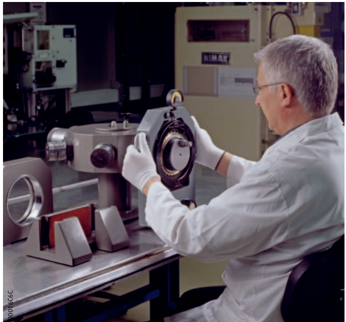
Figure 4 Positioning the enveloping circle gauge
