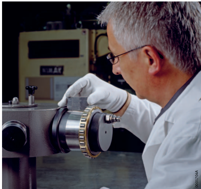
Figure 5 Measuring the distance to the shaft shoulder
