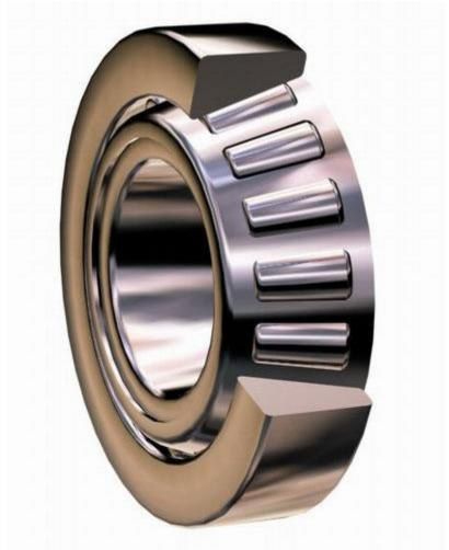
As the name implies, the rolling elements and raceways (of outer and inner rings) of these bearing are made with a tapered profile. These bearings can be separated into components, i.e. outer ring (cup), and the combined inner ring and roller assembly (cone).
