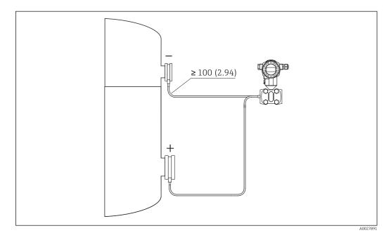
Due to the use of different process connections and capillary lines, it is essential that the device be designed/ordered using the "Applicator Sizing Diaphragm Seal" selection tool, which is available free of charge. Additional information can be found in the "Planning instructions, diaphragm seal systems" section → 🖺 89
