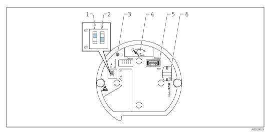
1 DIP switch for locking/unlocking parameters relevant to the measured value
