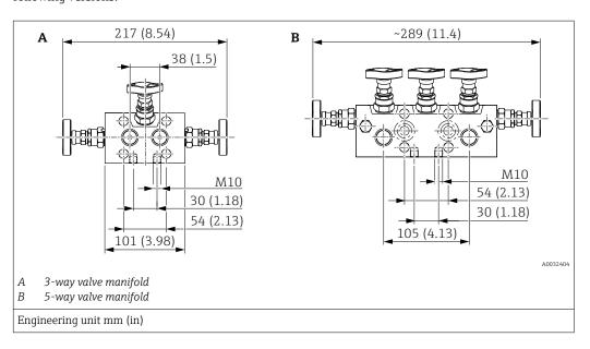
3-way or 5-way valve manifolds in 316L or AlloyC can be
