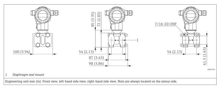
Process connections FMD78 with diaphragm seal
