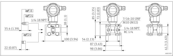
Engineering unit mm (in). Front view, left-hand side view, right-hand side view. Nuts are always located on the minus side.
