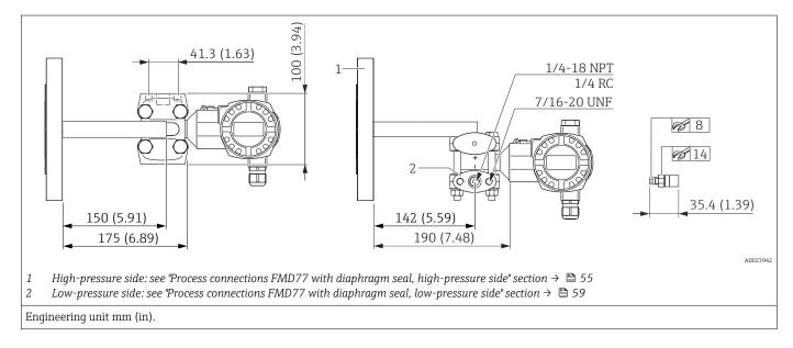
Process connections FMD77 with diaphragm seal
