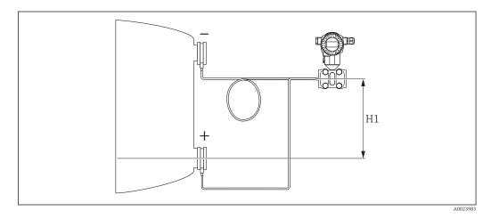
The maximum height difference is dependent on the density of the filling oil and the lowest pressure that is ever allowed to occur at the diaphragm seal on the positive side (empty container), see the following illustration:
