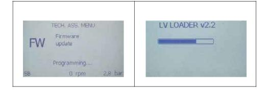
The programming starts. Wait until the end of the process and for the pumps' restart.
