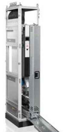
Optional cable panel installed inside the cabinet. ACS880-04 is pushed into the cabinet using a ramp and pedestal on wheels.
