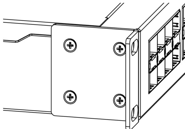
2. Place the device in the rackmount enclosure and align with the holes so that the device fits conveniently.
