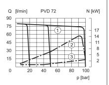
1 Flow rate - pressure curves, measured at 1450 rpm
