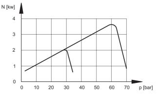
9 - PVE023 CHARACTERISTIC CURVES (values obtained with mineral oil with viscosity of 46 cSt at 40°C)
