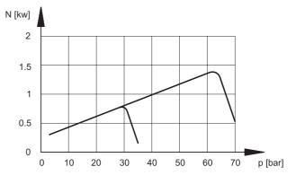
7 - PVE011 CHARACTERISTIC CURVES (values obtained with mineral oil with viscosity of 46 cSt at 40°C)
