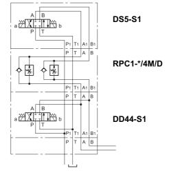
Example of circuit used to drive working units with fast approach, adjustable working speed and fast return.
