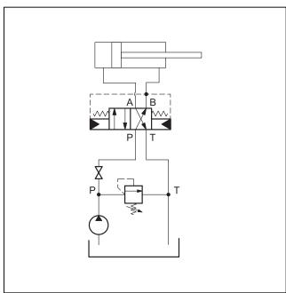
We suggest to use the circuit shown in the application example where, when the pump start to give flow the cylinder is ready to retract.
