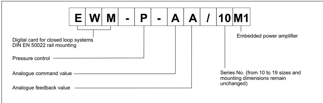
This module is useful for pressure control in very different applications. The output signal can control various kind of pressure valves, but the controller structure is optimized for pressure closed loop control system with typical pressure valves. An integrated power stage and high dynamic control loops (1 msec for pressure control and 0,167 msec for the current loop control) offers a simple solution.
