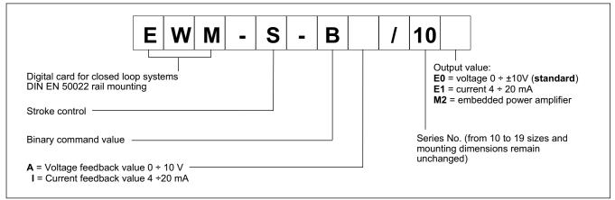
This module supports the simple point-to-point positioning with hydraulic drives. Two operating modes can be selected: stroke depending deceleration, that means the control gain will be adjusted with the parameters D:A and D:B, and NC mode, where the position value is generated from the following error.
