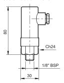
This indicator is a pressure switch sensitive to the filter input pressure, which switches an electric contact when the filter element has reached the clogging limit.
