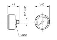
This indicator is a pressure gauge sensitive to the filter input pressure.
