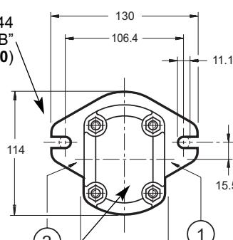
drainage port 1/4" BSP on reversible pump only
