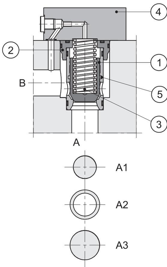
— Logic elements are cartridge valves suitable for installation in blocks or manifolds. They are available in five different sizes: ND 16 - 25 - 32 - 40 - 50 - 63.
