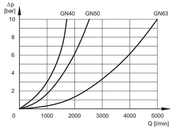
**4.2 - Flow control function with damping nose LC\*-QD**
