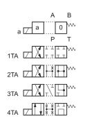
Type \*TC: 1 solenoid side B 2 positions (central + external) spring centering
