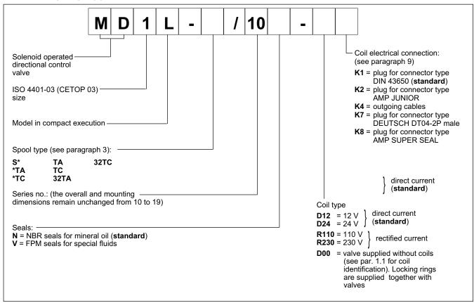
**NOTE**: The standard valve is supplied with phosphating surface treatment, black colour.
