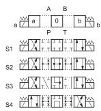
Type \*TA: 1 solenoid side A 2 positions (central + external) spring centering
