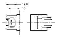
connection for AMP SUPER SEAL (two contacts) connector type code  ${\bf K8}$
