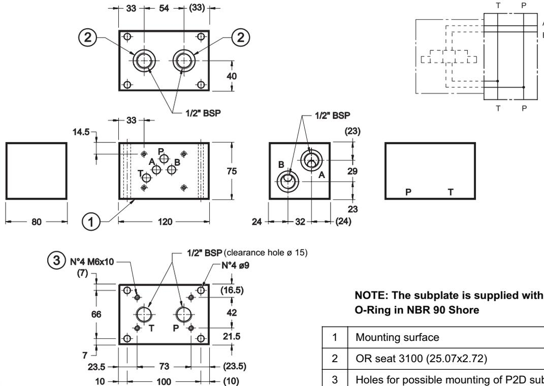
**NOTE: The subplate is supplied with O-Ring in NBR 90 Shore**
