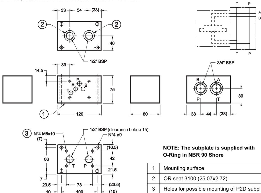
**NOTE: The subplate is supplied with O-Ring in NBR 90 Shore**
