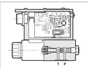
The PRED3G valve is a direct operated pressure control valve with integrated electric proportional control and mounting interface in compliance with ISO 4401 (CETOP RP 121H) standards.
