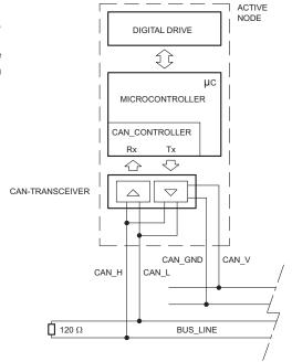
**N.B.**: insert a 120  $\Omega$  resistance on pin 4 and pin 5 of the CAN connector when the valve is the end-knot of the CAN network.
