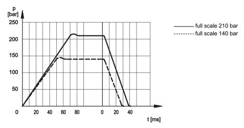
**NOTE**: Response times are obtained by using valves with a full scale of 140 and 210 bar, with an input flow rate of 2 l/min and a pressure oil volume of 0,5 lt. The response time is affected both by the flow rate and the oil volume in the pipework.
