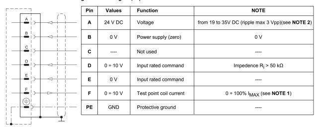
**NOTE**: If only one input signal is available (single-end), then the pin B (0V power supply) and the pin E (0V reference signal) must be connected through a jumper and both connected to GND, electric panel side.
