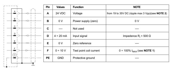
**NOTE for the wiring:** connections must be made via the 7-pin plug mounted on the amplifier. Recommended cable sizes are 0,75 mm<sup>2</sup> for cables up to 20 m and 1,00 mm<sup>2</sup> for cables up to 40m, for power supply. The signal cables must be 0,50 mm<sup>2</sup>. A suitable cable would have 7 cores, a separate screen for the signal wires and an overall screen.
