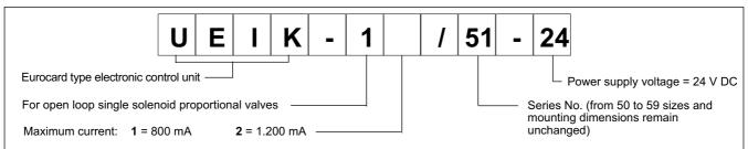
The UEIK-1\* card is an electronic control unit Eurocard type for open loop single solenoid proportional valves.
