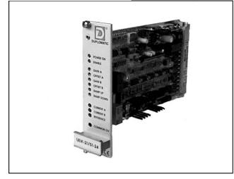
UEIK-2\* ELECTRONIC CONTROL UNIT FOR OPEN LOOP DOUBLE SOLENOID PROPORTIONAL VALVE SERIES 51
