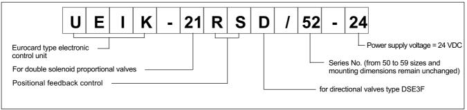
The UEIK-21RS card is an electronic control unit Eurocard type for closed loop control of double solenoid proportional valves with positional feedback control.
