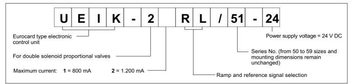
The UEIK-2\*RL card is an electronic control unit in Eurocard format for open loop control of double solenoid proportional valves, with selection in sequence of four different reference and ramp time regulation signals.
