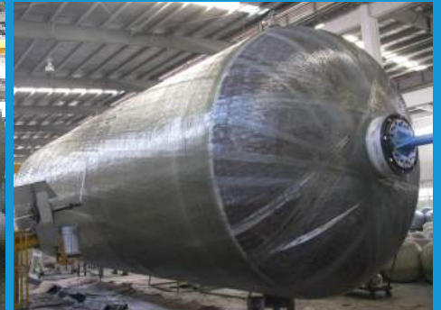
Computer Controlled Filament Winding
