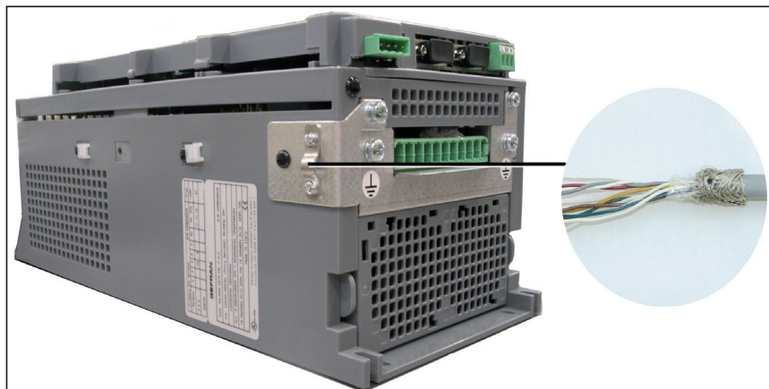
Figure 7.2.4: Connection of shielding (recommended)
