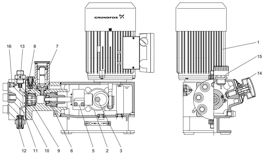
**Fig. 22** Sectional drawing, DMH model 280
