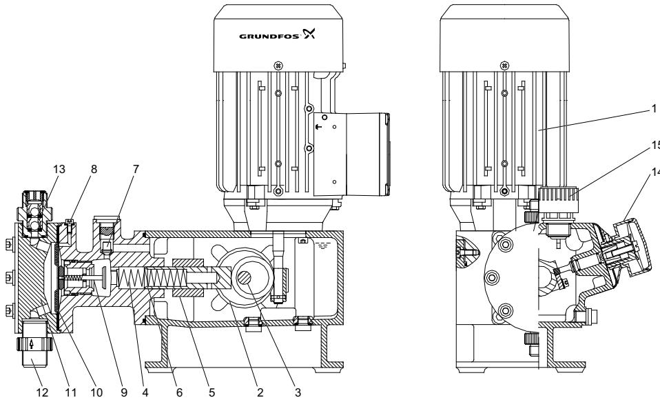
**Fig. 17** Sectional drawing, DMH models 251, 252
