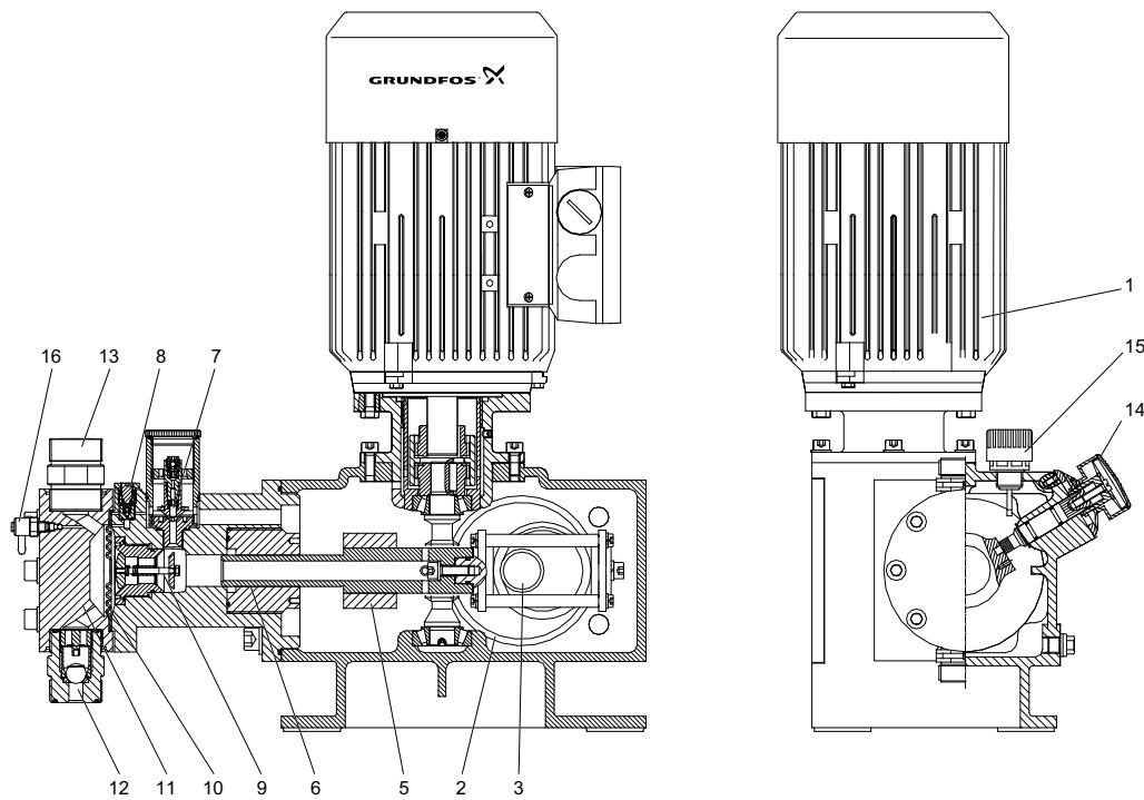
**Fig. 24** Sectional drawing, DMH models 285, 286, 287
