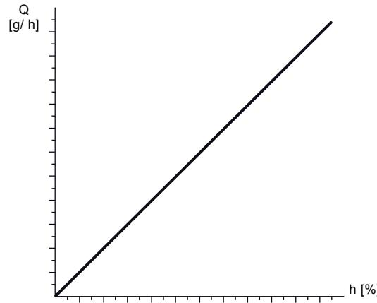
**Fig. 3** Relation of stroke length and capacity
