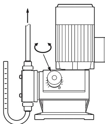
**Fig. 2** Capacity control by stroke length adjustment knob
