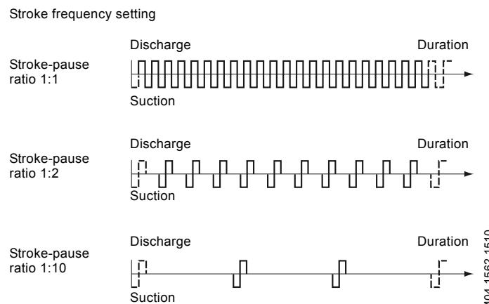
**Fig. 7** Relation of stroke frequency setting - capacity
