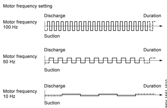
**Fig. 5** Relation of motor frequency setting - capacity
