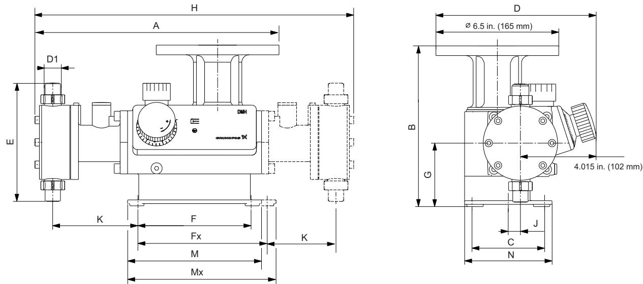
**Fig. 25** Dimensions, DMH models 251 to 281
