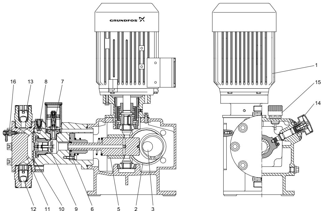
**Fig. 23** Sectional drawing, DMH models 283, 288
