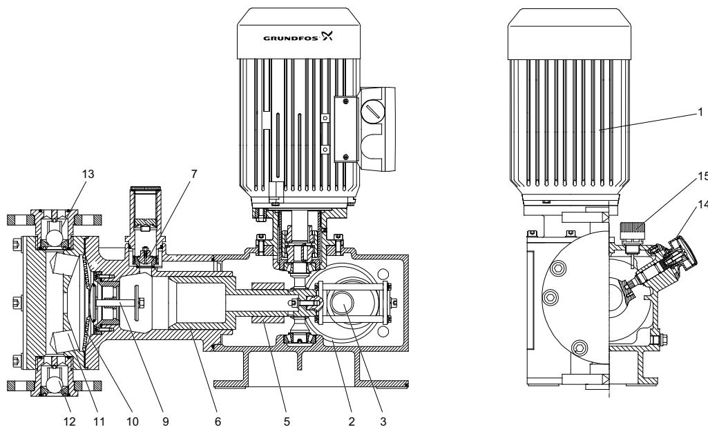
**Fig. 21** Sectional drawing, DMH model 257
