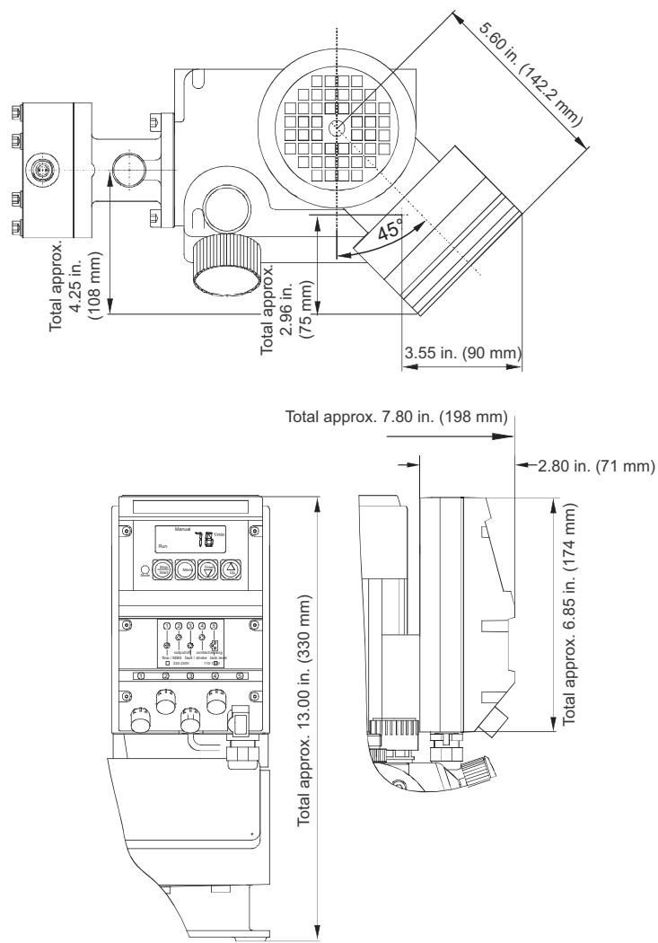
**Fig. 27** Dimensions, AR control unit (mounted on DMH)
