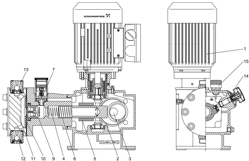
**Fig. 19** Sectional drawing, DMH model 254
