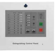
The GST301 is standalone gas extinguishing control panel, provides 2 conventional detection zones to achieve double knock control, and an additional standard fire detection zone for other areas. The Duty and Standby Cylinder control can be automatic and manual controlled, with
