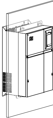
Figure 3-11 Embedded installation effect of the MD380 (sheet metal housing)
