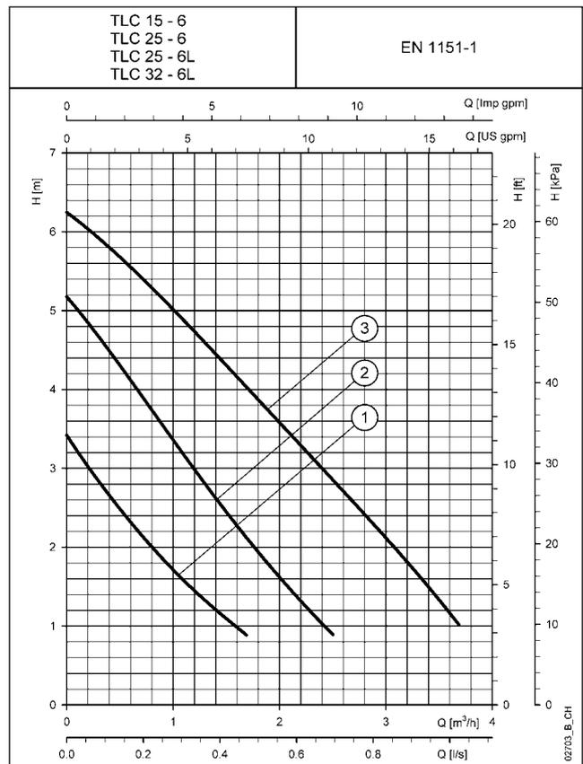
These performances are valid for liquids with density  $\rho = 1.0 \text{ Kg/dm}^3$  and kinematic viscosity  $\nu = 1 \text{ mm}^2/\text{sec}$ .
