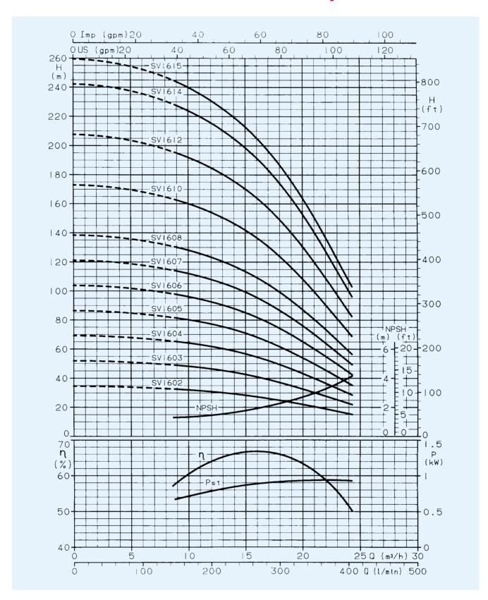
These performances are valid for liquids with density  $\rho=1.0\ kg/dm^3$  and kinematic viscosity  $\gamma=1\ mm^2/sec.$
