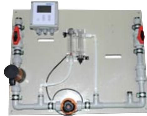
Version dedicated to the **measurement of chlorine** with a potentiostatic probe.
