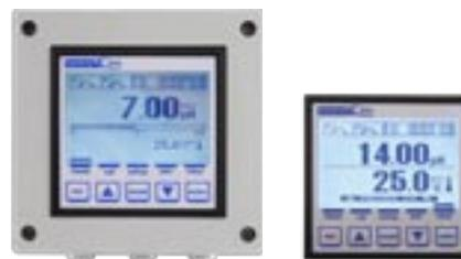
The **multi-colour backlit function, with four different colors**, makes it easy to interpret what function the controller is in even in poor light conditions.
