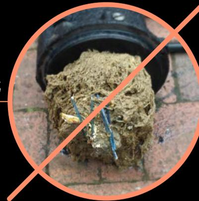
*Clogged pump, without grinding system*
