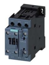
power contactor, AC-3e/AC-3, 17 A, 7.5 kW / 400 V, 3-pole, 24 V DC, auxiliary contacts: 1 NO + 1 NC, screw terminal, size: S0  $\,$
