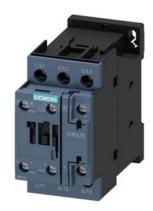
power contactor, AC-3e/AC-3, 32 A, 15 kW / 400 V, 3-pole, 110 V AC, 50 Hz, auxiliary contacts: 1 NO + 1 NC, screw terminal, size: S0  $\,$
