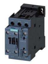
power contactor, AC-3e/AC-3, 32 A, 15 kW / 400 V, 3-pole, 24 V DC, auxiliary contacts: 1 NO + 1 NC, screw terminal, size: S0
