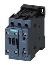
power contactor, AC-3e/AC-3, 38 A, 18.5 kW / 400 V, 3-pole, 24 V DC, auxiliary contacts: 1 NO + 1 NC, screw terminal, size: S0  $\,$
